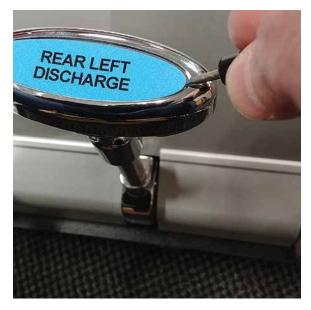
1. Using a small flathead screwdriver, remove the label from the top of the T-handle. Be carful not to damage the chrome that will be visible after the repair is complete.
