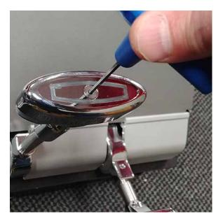
10. Making sure that the springs are present and properly seated, tighten the screw until it stops. An extra screw has been provided in case the original was stripped during removal.
