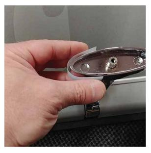
6. Remove liner from 1 of 2 pieces of polyethylene tape. Install onto base as shown - flush with top edge. Press down firmly or burnish to ensure good adhesion.
