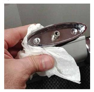
5. Clean and wipe the outer surface of the T-handle base with isopropyl alcohol or equivalent.
