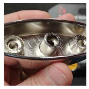
9. Place the T-handle cap back onto the assembly being very careful to seat the top of the springs into the recesses on the underside of the casting. This can be difficult at first.
