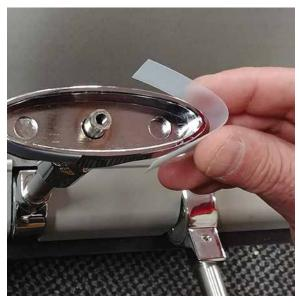
7. Using second piece of ultra high molecular weight polyethylene tape, repeat step 6 on other side of T-handle base.
