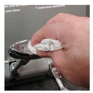
11. Clean and wipe the label recess with isopropyl alcohol or equivalent.
